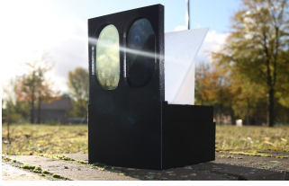
Figure 13: The LuxLink transmitter: light is reflected on the white surface and passes through the LCDs.
