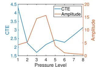
Figure 6: The CTE and amplitude change along with pressure levels.
