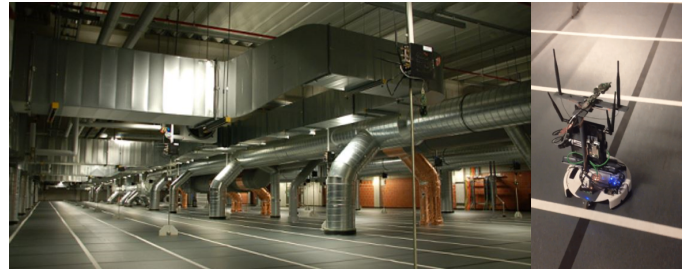
Fig. 5: Wilab2 testbed setup showing static Wi-Fi nodes on the left and mobile robots to the right
