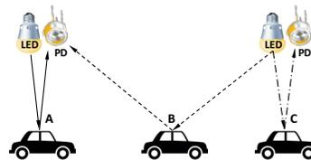
Fig. 1. The concept of passive localization with smart lights.
