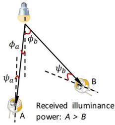
Fig. 2. The Lambertian model.
