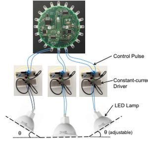
Fig. 12. Our testbed with the front-end Shine++
