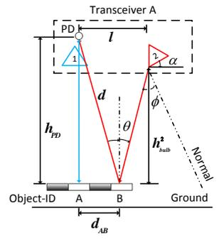
Fig. 10. Illustration of the geometric model used to remove the ISI
