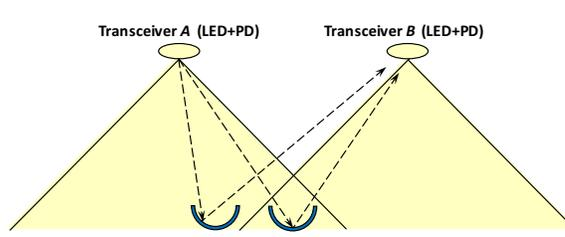
Fig. 5. The problem of unique signature when each transceiver has a single beam (the object has many tiny reflective surfaces tiled at different angles (kind of ‘retro-reflector’) to improve the coverage)
