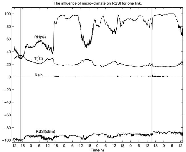
Fig. 5. Influence of the micro-climate on RSSI against time, for receiver 1 and transmitter 13 (23 m apart, low SNR regime).
