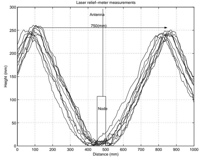
Fig. 2. The dimensions of the ridges with a node schematically drawn. Ridge height 25 cm, Ridge width 75 cm, Antenna height 11 cm and Total node height 29.5 cm.
