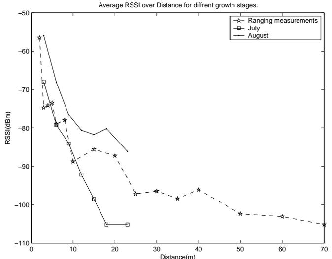
Fig. 3. Signal strength vs. distance.
