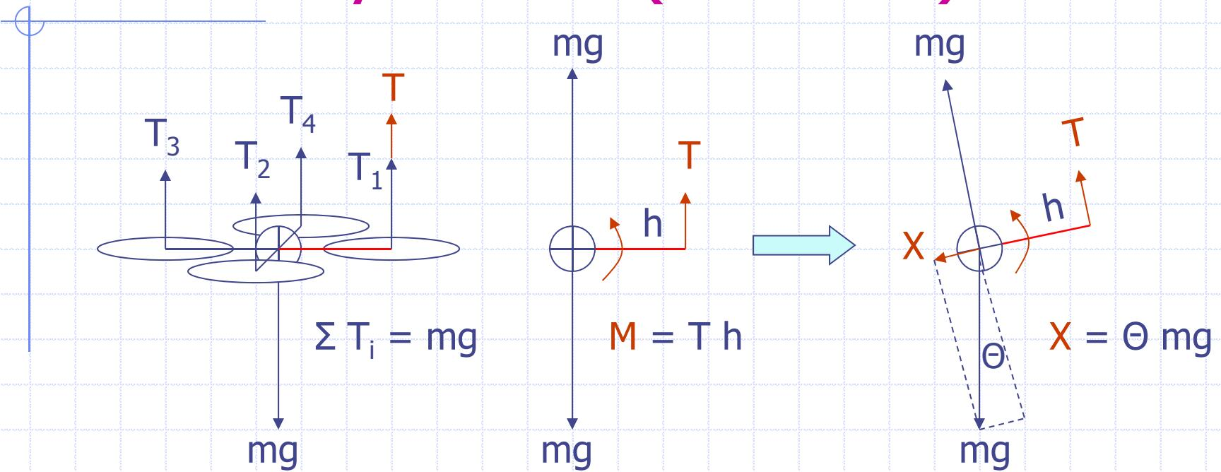
$T_i$  = rotor thrust =  $f(\Omega_i)$
