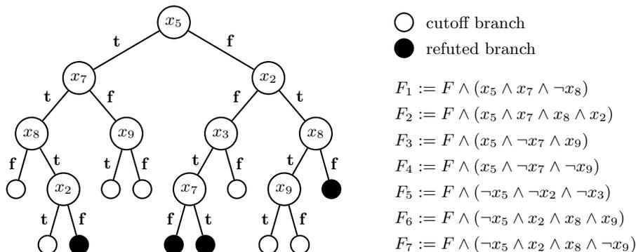
**Fig. 1.** A partition of a CNF formula  $F$  into seven subformulas  $F_i$ . The binary search tree on the left is constructed by a lookahead solver. It shows in the internal nodes the decision variable, and on the edges the truth value of a branch. Black nodes represent refuted branches, while white nodes are cutoff branches. The decisions of cutoff branches yield a cube of assumptions that together with  $F$  forms a subformula  $F_i$ .
