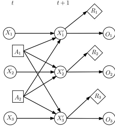
Figure 1: Two-stage DBN for the adapted fire fighting problem, where  $X_i = \{0, 1, \dots, k-1\}$ ;  $O_i = \{0, 1, \dots, l-1\}$ .
